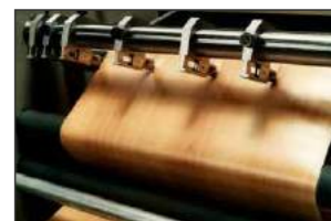
SYSTEM CI CIA NO AMI YLETKOWYMI SLITTING SYSTEM WITH RAZOR TYPE KNIFE
